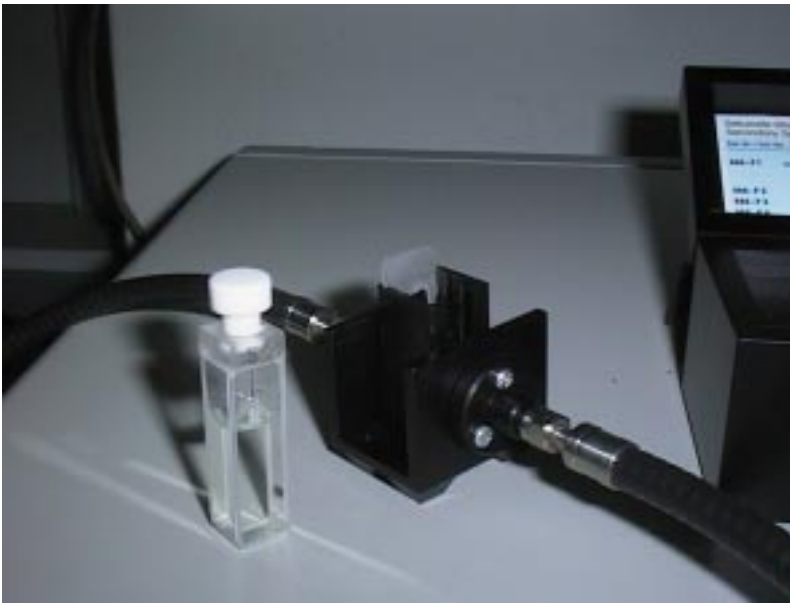
NaNO 2 solution cell for false light test, cell holder and monofibres.
