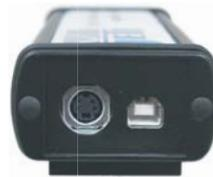
Connector for USB BUS and External trigger
