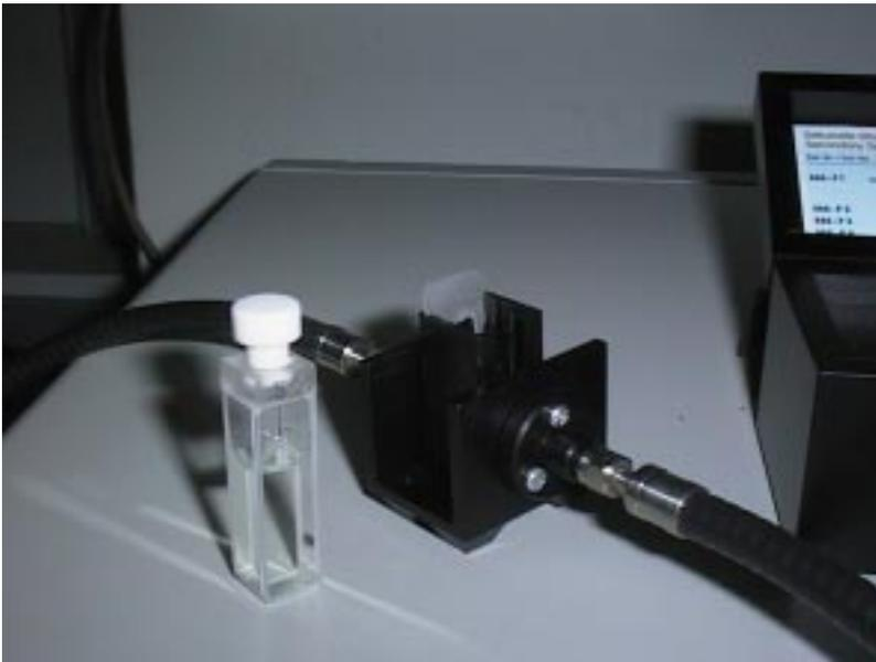
NaNO<sub>2</sub> solution cell for false light test, cell holder and monofibres.
