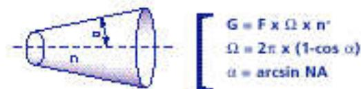
$$\begin{aligned} G &= F \times \Omega \times n^2, \\ &= 2\pi \times F \times (1 - \cos \alpha) \times n^2, \\ &= 2\pi \times F \times n^2 \times (1 - \sqrt{1 - NA^2}) \end{aligned}$$
