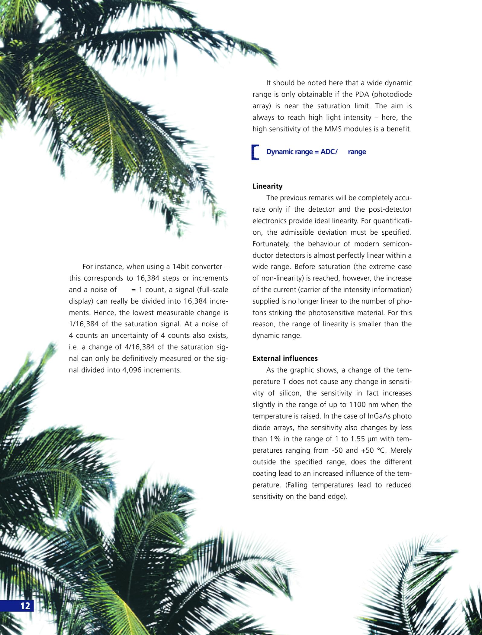
It should be noted here that a wide dynamic range is only obtainable if the PDA (photodiode array) is near the saturation limit. The aim is always to reach high light intensity – here, the high sensitivity of the MMS modules is a benefit.
