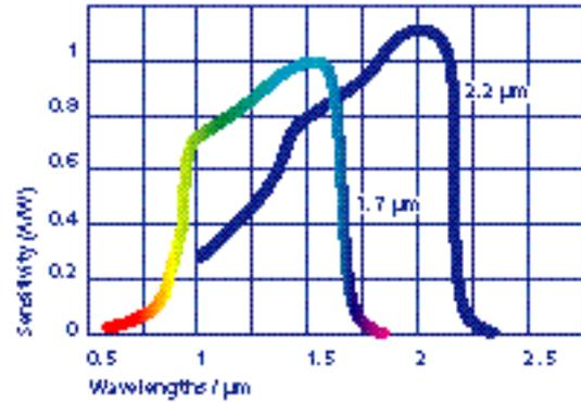
Spectral sensitivity of standard-InGaAs (1.7 μm) and extended-InGaAs (2.2 μm)
