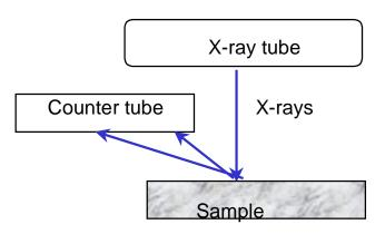
Non-contact layer thickness measurement
