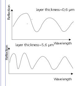
Phase evaluation of thin layers 0,5µm -1µm
