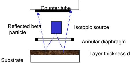
Non-contact thickness measurement of layers whose atomic number differs substantially from the substrate material.
